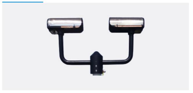
ZDM100 Disdrometer is a laser instrument that measures the drop size distribution falling hydrometeors. It can also monitor rainfall types, visibility, radar reflectivity and other parameters. It is widely used in the field of hydrometeorology.
