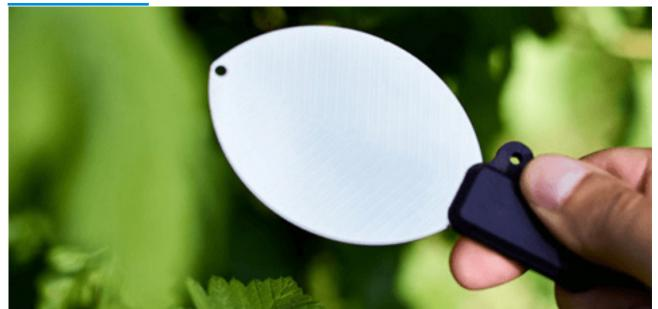
ZLW-2 leaf wetness sensor can accurately measure the humidity of the leaf surface, and can monitor the trace water or ice crystals on the leaf surface.
