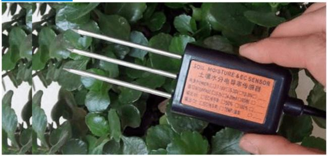
ZSTM-3 soil sensor which can measure soil moisture & EC & temperature, provided with high accurate and high sensitive. It is an important tool to observe and study the occurrence, evolution, improvement and the dynamics water of saline soil
