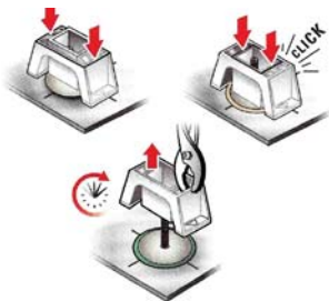
Step 1 - Mount the sensors with included mounting studs
