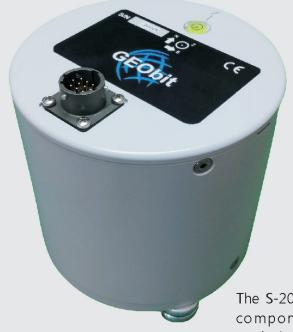
The S-20 sensor series is a three component velocity output equivalent seismic sensor for local and regional seismicity monitoring. The sensor range is 20sec to 50Hz flat to velocity. The sensitivity is 1500V/m/s. The instrument is a perfect solution where near broad band seismic sensor is required.
