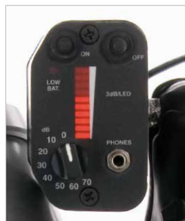
LED display and sensitivity dial
