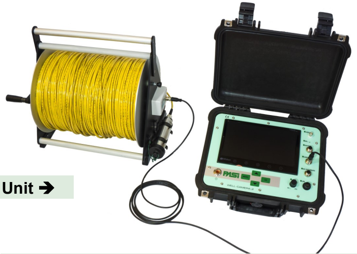
← ASPO 50: with 50m of fiberglass cable & Teflon adapter for Well-Camera Head Aspo dim: 51cm x 62cm x 22 cm - Weight: 5,55 kg Teflon adapter: Ø 4,2 cm x 12 cm
