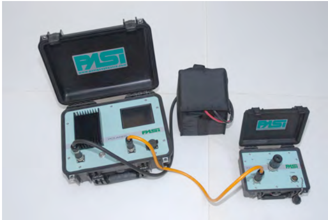
How to connect POLARES to a MUX for testing with special test connector
