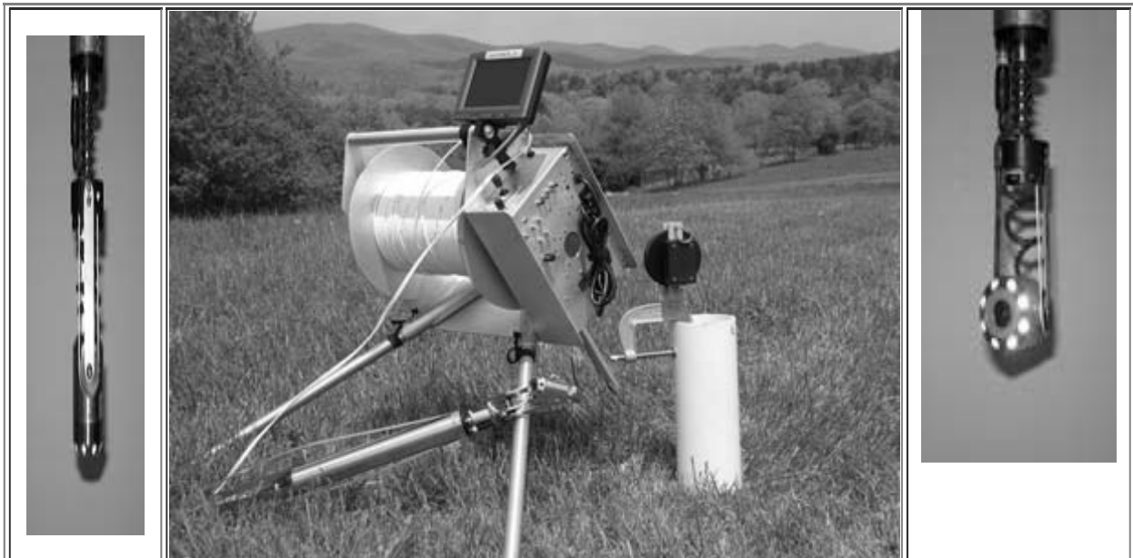
Pan and Tilt attachment with the standard stainless steel camera and centralizer assembly
