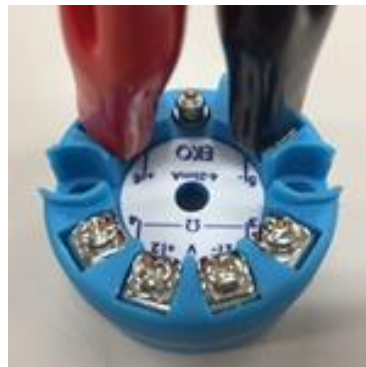
Figure A-7. Connection between the Signal Converter and Configurator Cable
